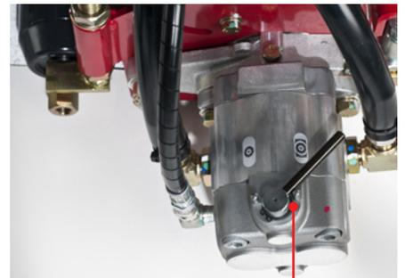
Reel Motor shut-off valve
